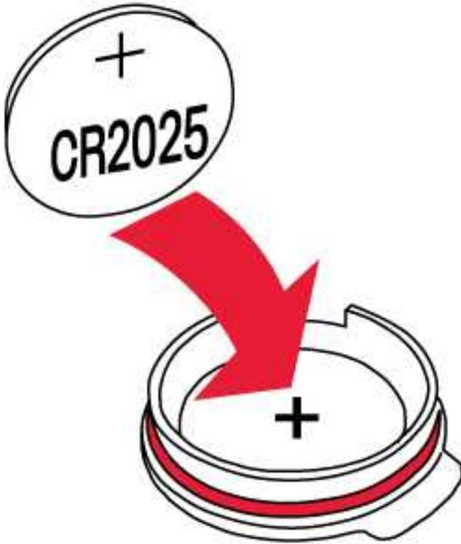
4. Make sure the red sealing ring is in place, clean and intact. If the sealing ring is damaged, replace it with a new one\*.
