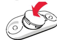
1. Lever the battery cover open by using the clip on the strap.
