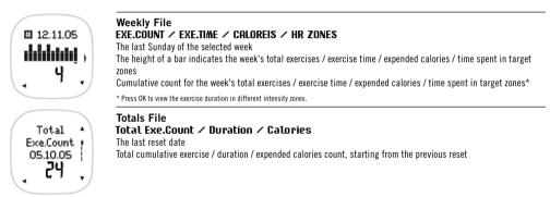
To empty the Totals File, press DOWN until **Reset Total Counters?** is displayed. Press OK and select the information you wish to erase. **ARE YOU SURE?** is displayed. Confirm deletion with **YES**.
