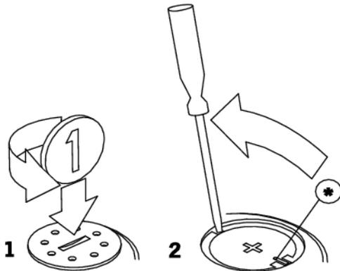
1. Open the battery cover with a coin by turning it from CLOSE to OPEN.
