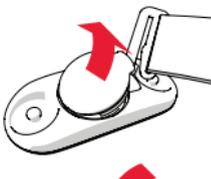
1. Lever the battery cover open by using the clip on the strap.
